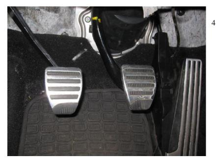
41.) With the AFP Adjuster set to roughly around 70% (doesn't need to be exact) and the return spring still sitting loose have a look at how high the new clutch pedal is relative to the brake pedal height. Using your Needle nose pliers turn the clutch rod Right (Counter Clockwise) until the clutch pedal is leveled up with the brake pedal height while leaving the 2pc arm adjustment centered.
