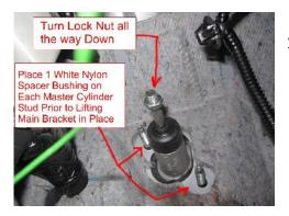
22.) Take the two white nylon spacer bushings included in the parts bag and place one over each of the master cylinder studs. These hold the bracket up over the firewall padding. Spin the lock nut on the clutch rod all the way down lightly by finger.
