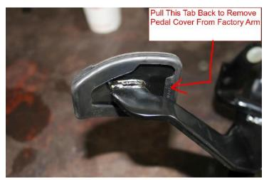
16.) Next carefully pull the pedal cover from the factory pedal starting at the back by rolling the rubber lip back out of the way while carefully pulling the cover off.
