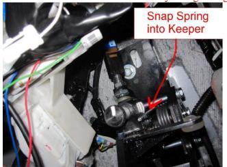
Photo Note: V2 Assemblies have only a single long slot.
