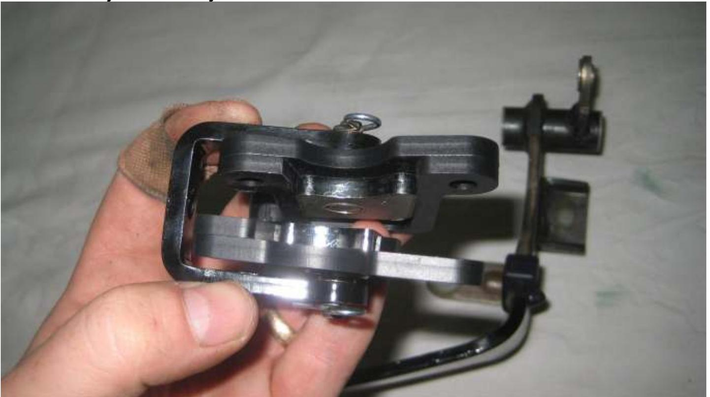
. You will need to guide the assembly in place around the switch pad mounts in order to get it fully seated against the pivot tube at the top.
