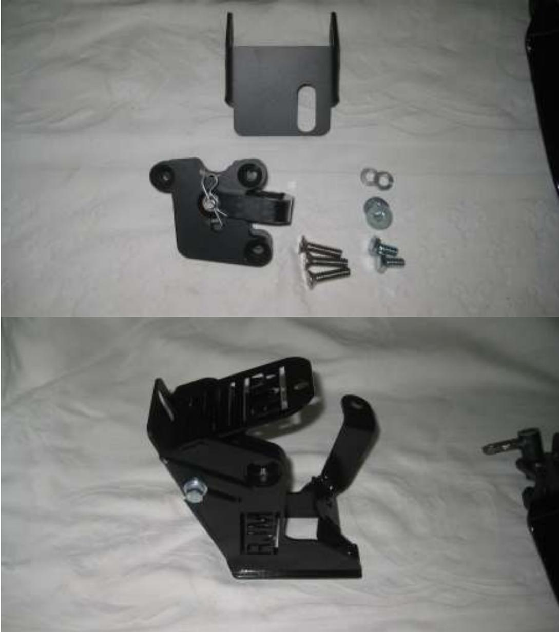
**NOTE: Rev 2 Top Bracket Design has removed the second bolt on the top left side of the bracket and is replaced with a single long bolt and sliding nut that clamps the bracket from the much easier to access top right corner.**
