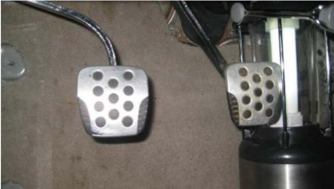
Once you're satisfied with the initial position of the clutch pedal go back and adjust the upper switch so that it too gets just depressed by the pedal while fully at rest but does not bottom out the switch and hold the clutch pedal from returning all the way up.
