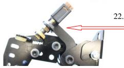
22.) Next install the Brown Cruise Control switch into the upper switch mount followed by an oem switch lock nut. Set this switch so there is an equal amount of threading on either side of the metal tab and tighten both lock nuts using your 14mm & 17mm wrenches together.
