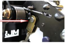
29.) Now get a Deep 12mm socket, long extension and ratchet ready for this step. Moving the bracket up or down alters the angle of the clutch rod which needs to push straight in/out of the master cylinder. Move the bracket to where the rod looks to be going straight into the master cylinder and tighten the upper right stud nut firmly, followed by tightening the lower left stud nut firmly and finish by tightening the upper dash bolt. (*See Reference Photos at Steps 26 & 27*)
