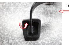
16.) Next carefully pull the pedal coverfrom the factory pedal starting at the top left corner by rolling the rubber lip back out of the way and pulling the cover off.
