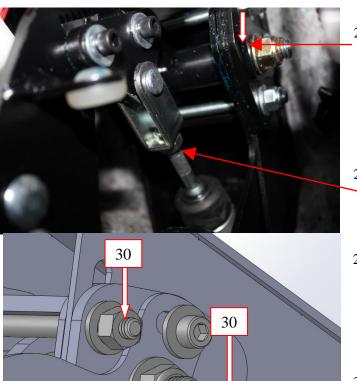
27.) Pull the sliding center section of the pedal assembly down towards the floor as far as it'll go.
