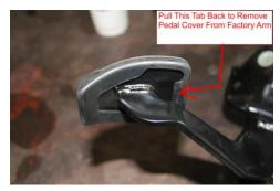
14.) Next carefully pull the pedal cover from the factory pedal starting at the back by rolling the rubber lip back out of the way while carefully pulling the cover off. It'll just peel off.
