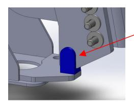
18.) Take the Blue Stop bumper and press it thru the hole on the new pedal arm as shown so the flat face is on the Left Side.
