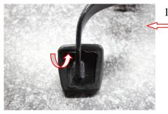
16.) Next carefully pull the pedal coverfrom the factory pedal starting at the top left corner by rolling the rubber lip back out of the way and pulling the cover off.
