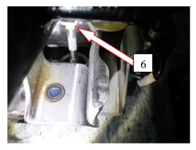
6.) Next Locate the Clutch Rod going into the master cylinder that connects to the Factory Clevis End as shown in the photo. There is a Lock Nut behind the clevis on the threaded section of the master cylinder rod. Using a 12mm Open End Wrench, come in from below the pedal arm and find the best wrench position to get onto the flats of the nut to turn it <u>Clockwise</u> and loosen the nut - Just need to turn it enough to break it free so the clevis end can be removed later.
